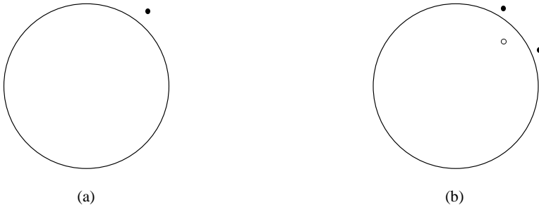
Fig. 2.2. (a) One electron is excited outside the Fermi sea with total energy \epsilon . (b) The extra electron has scattered off an electron in the Fermi sea leaving a hole and both electrons lie outside the Fermi sea. The energy and momentum of the configuration shown in (b) must be equal to that in (a).
